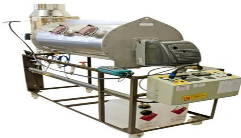
Figure 4: Photographic view of a laboratory-scale cylindrical combustion chamber with burner assembly and control unit
