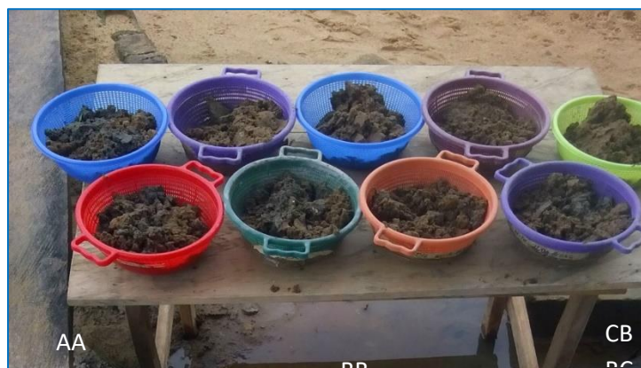
Fig 2.4. The experimental setup for the study showing treated soil samples in perforated plastic containers.
