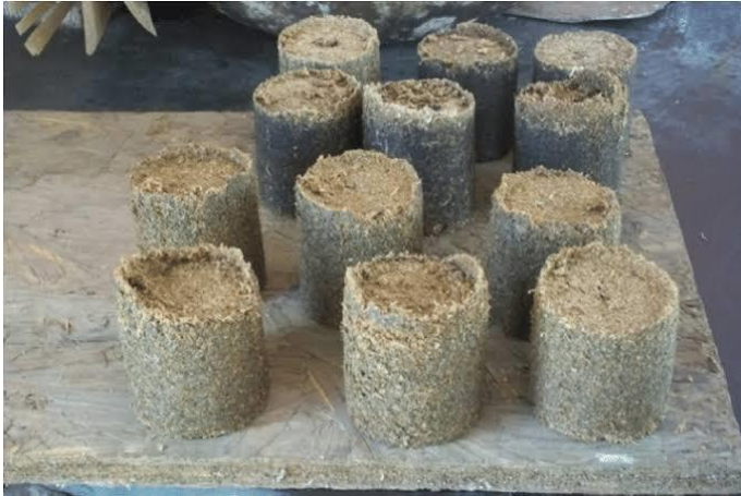
Plate 1: Sample of briquettes prepared from sheanut-shell.
