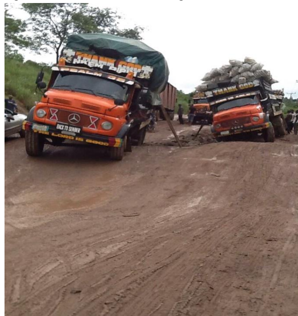
Fig.3: Breakdown of trucks caused by swelling soil.
