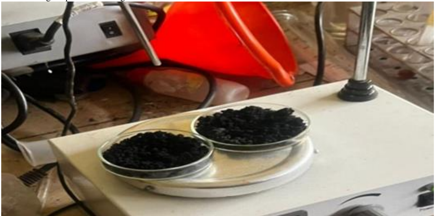
Figure 2. Activated and carbonized palm kernel shell The physicochemical properties (moisture, ash, pH, pore volume) of the adsorbent were analyzed.
