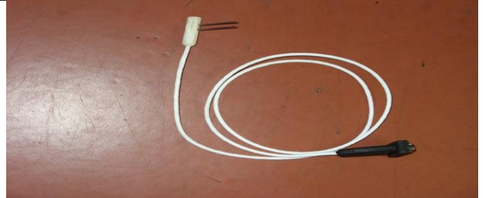
Figure 20. Dual-needle sensors for volumetric specific heat capacity and diffusivity measurements (30 mm).
