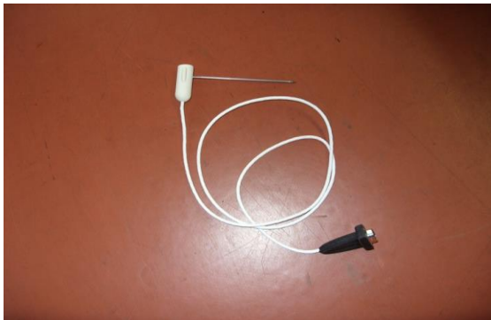
Figure 19. Extended single-needle sensors for thermal conductivity and resistivity measurements (10 cm) for use in hard materials.
