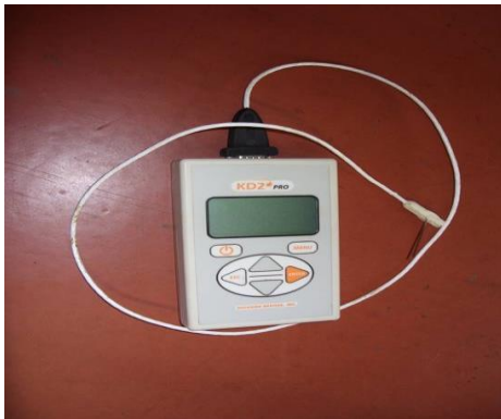
Figure 18. Single-needle sensors for thermal conductivity and resistivity measurements (6 cm) for liquids.
