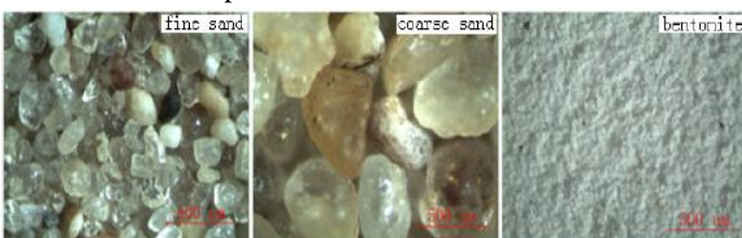
Figure 2. Micrographs of dry sand and bentonite grains.
