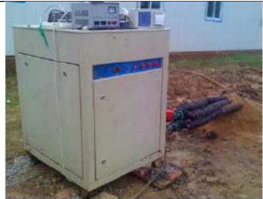
Figure 4. A part of view of field tests of the thermal performance of the BHEs Results and Discussion.
